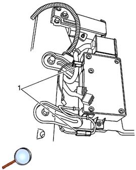
4. Disconnect the cellular antenna and the navigation radio antenna connectors (1).
